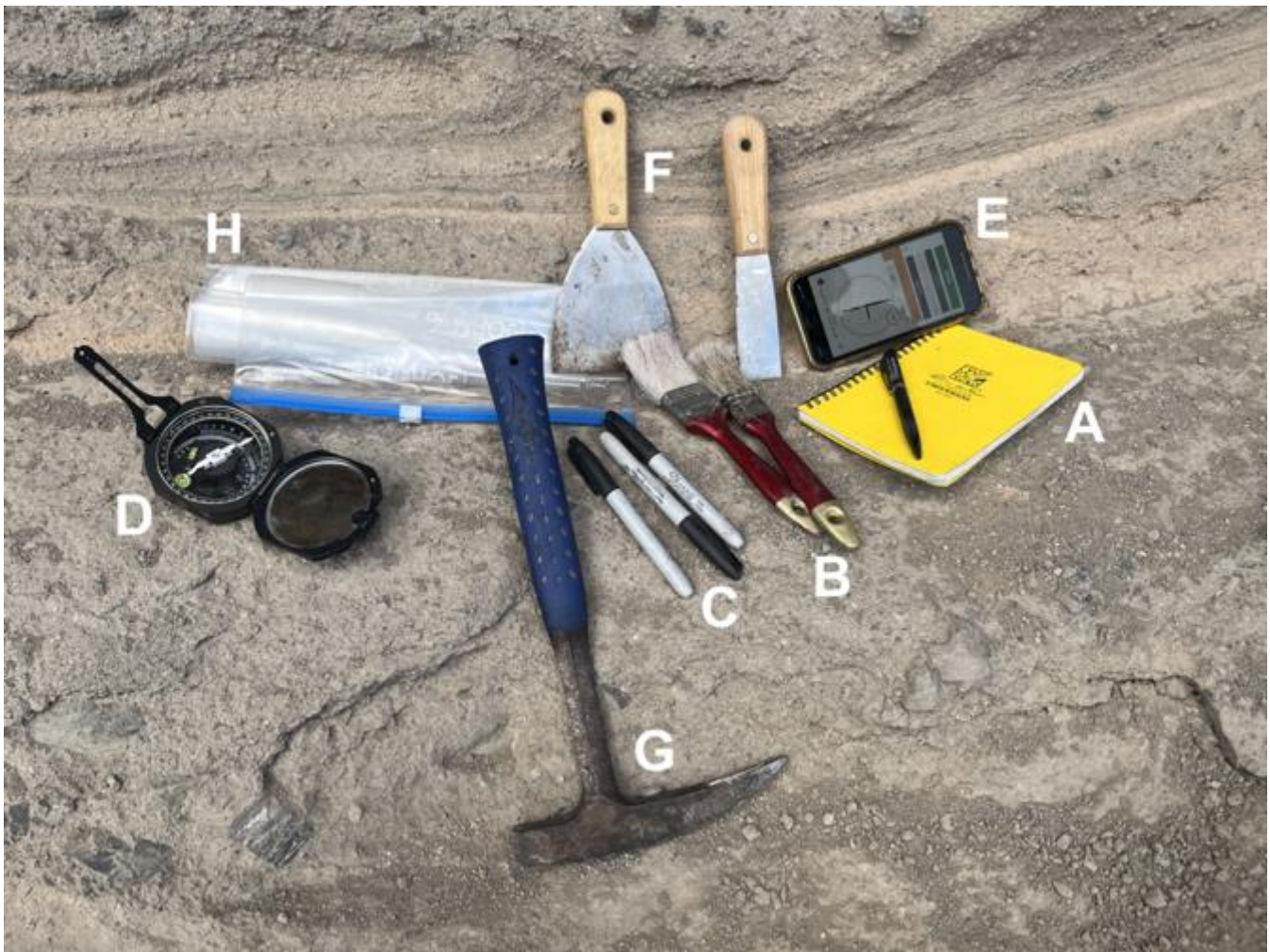
265 Figure 7: Key equipment for paleomagnetic sampling of pyroclastic deposits: [A] Field notebook, [B] brushes of various sizes for cleaning rock samples before labeling, [C] permanent markers for labeling, [D] example of a geological compass-clinometer for orienting samples, [E] example of a smartphone compass-clinometer app that can also be used for sample orientation, [F] metal spatulas of varying sizes for cleaning the outcrop and the samples, 270 [G] geological hammer/pick for cleaning the area around the sample and removing the sample from the outcrop, [H] cloth and plastic sample bags for organizing oriented samples.
