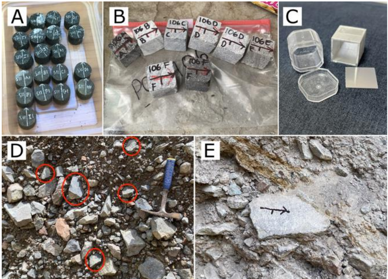
235 Figure 6: Photos showing important paleomagnetic sample and specimen characteristics. [A] example of 25 mm diameter, 25 mm-long cylindrical rock specimens, [B] 2 x 2 x 2 cm rock cube specimens, [C] specialized plastic and metal boxes for collecting 2 x 2 x 2 cm cubic samples of ash matrix, [D] PDC outcrop with several viable hand samples highlighted, [E] example of an ideal hand sample, note the flat face of rock that is ideal for measuring and labeling.
